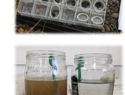
• Soil aggregates are immersed in water and soil stability can be estimated
