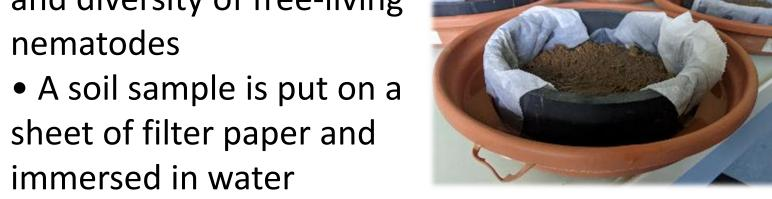
Nematodes swim through the filter paper and are extracted and counted
